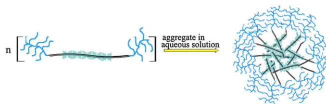
Scheme 2. Schematic diagram of self-assemblies formed by the PR-based triblock copolymer in aqueous medium.
